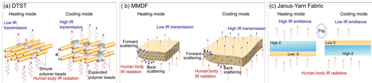
Figure 1. Schematic illustration of the working principle behind (a) Dynamic Transmittance Switch Textile (DTST), (b) Metallic Microparticle-based Dynamic Fabric (MMDF), (c) Janus-yarn fabric.
