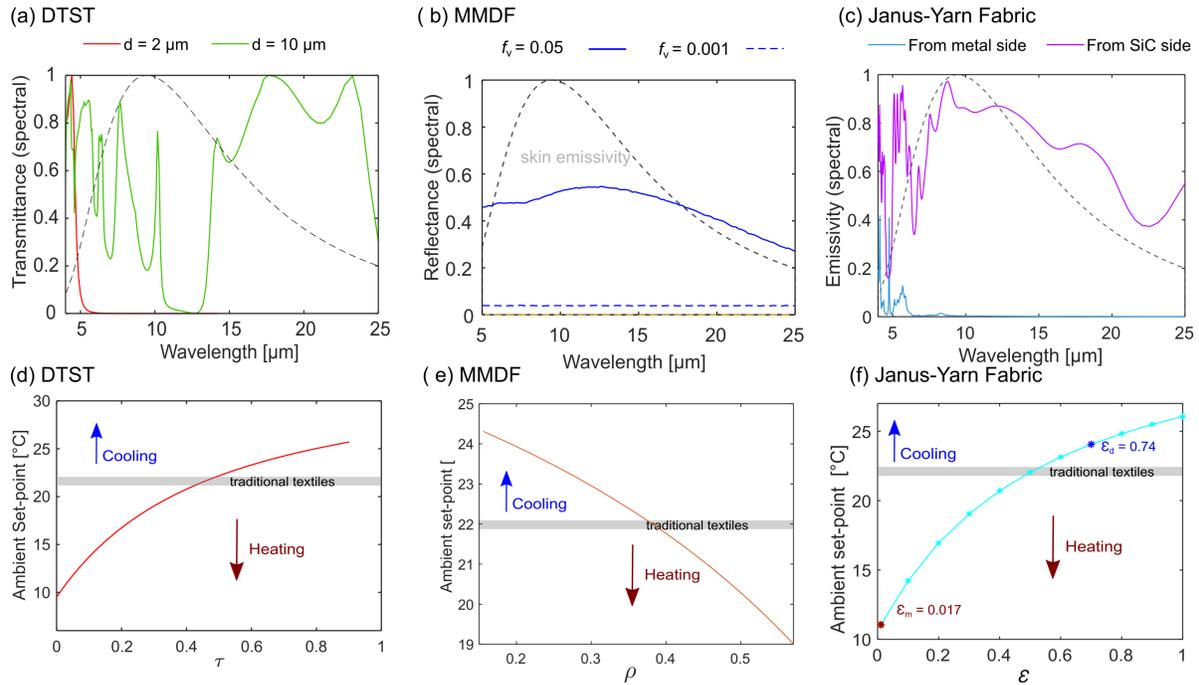
Figure 3. (a) Spectral transmittance of DTST. (b) Spectral reflectance of MMDF. Spectral emissivity of Janus-yarn fabric. (d) Ambient setpoint temperature of DTST as a function of transmittance  $\tau$ . (e) Ambient setpoint temperature of MMDF as a function of reflectance  $\rho$ . (f) Ambient setpoint temperature of Janus-yarn fabric as a function of transmittance  $\epsilon$ .
