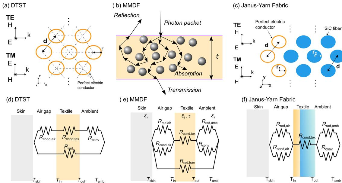
Figure 2. The schematic of simulated model for the IR response: (a) DTST, (b) MMDF and (c) Janus-yarn fabric; and for heat transfer (d) DTST, (e) MMDF, and (f) Janus-yarn fabric, respectively.
